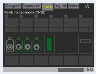
Figure 8: Status menu screen displays instrument, fluid container, and column status.
