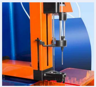
**Figure 2:** The robotic needle arm allows accurate and highly reproducible pipetting and enables fully automated cell separation with consistent results.
